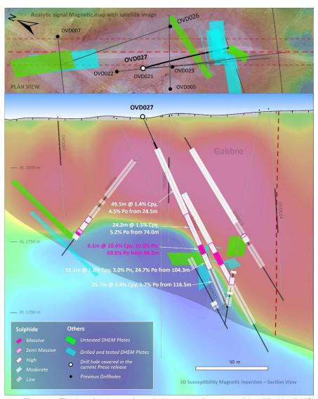
Figure 2. The longitude section of all conductive plates identified by DHEM<sup>6</sup>
