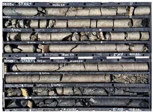
Photo 1. The massive sulphide intersection in drillhole OVD027
