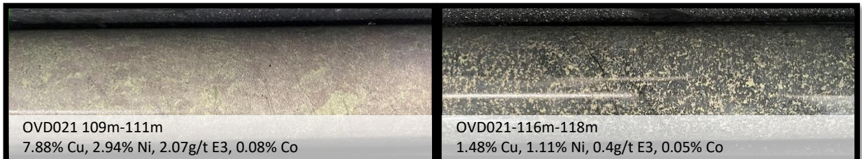
Photo-1. Massive sulphide and matrix/net textured sulphide interceptions from OVD021 with details. Image represents the style of mineralisation in short segments from longer assay intercepts, given in the figure.
